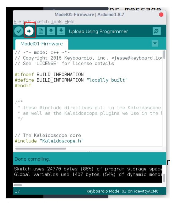
If the process is successful, Arduino will tell you that in the status area. Some keyboards may also use LEDs to report their results. For example, the Model 01's LED's flash red across the board as the firmware is installed, and then the "LED" key glows blue.
